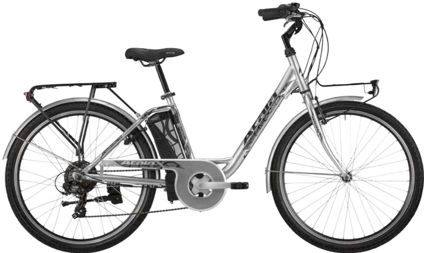
**FRAME** Hi-Ten Tig 26", easy access, internal cables, side mount battery
