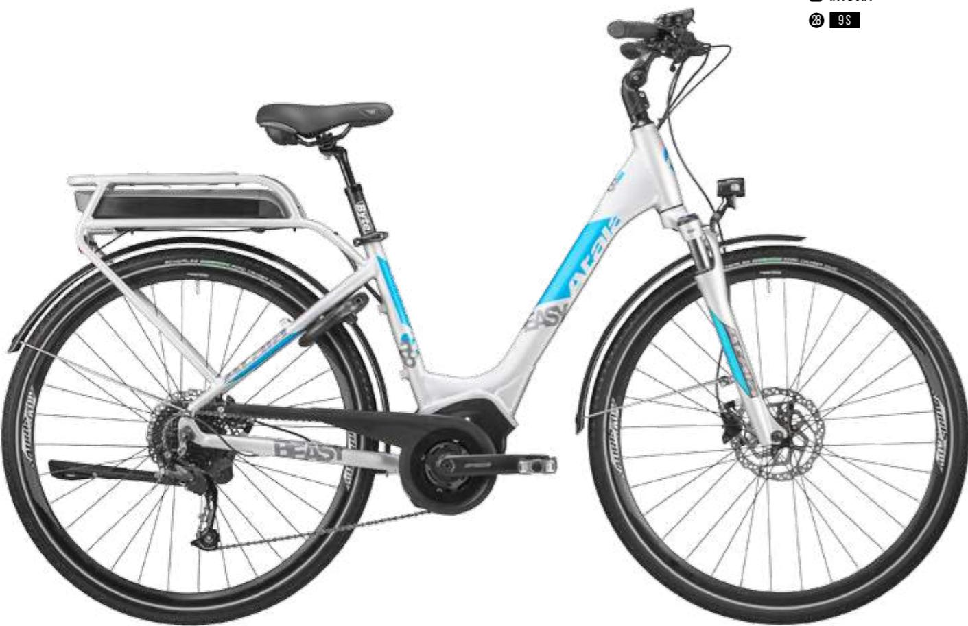
**FRAME** Alu 700C, easy access, custom tubing, Integrated carrier, Internal routing, Forged interface
