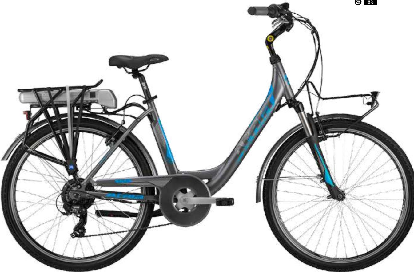
**FRAME** Alu. Formed 26", easy access, internal cables
