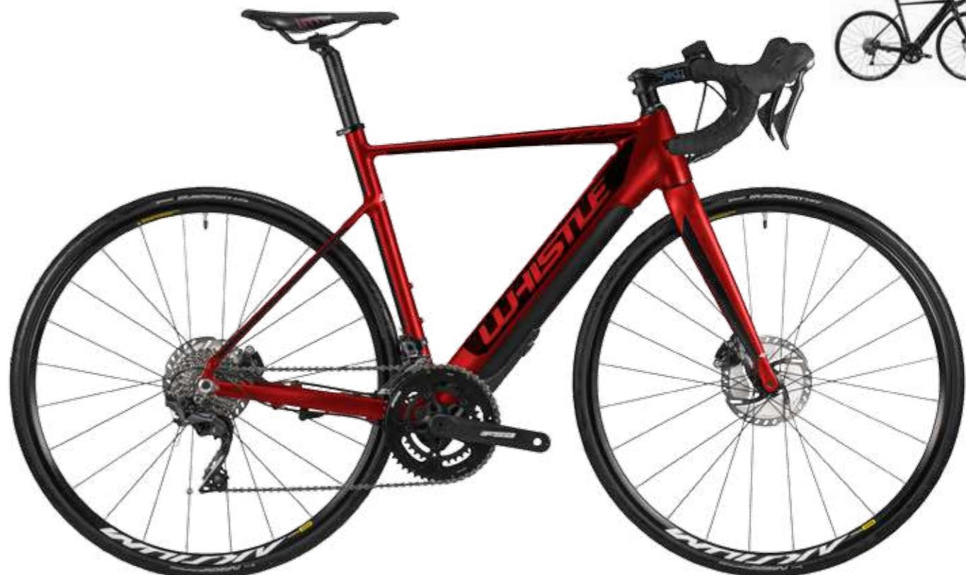
**FRAME** Alu, hydroformed, smooth welding. Flat mount, tapered, 12x142 mm
