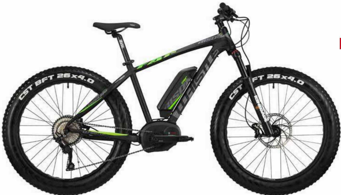
**FRAME** Alu 26" FAT, hydroformed, tapered, 12x197 mm,
