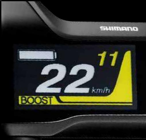
LCD screen with gear, assistance level, range and speed.
