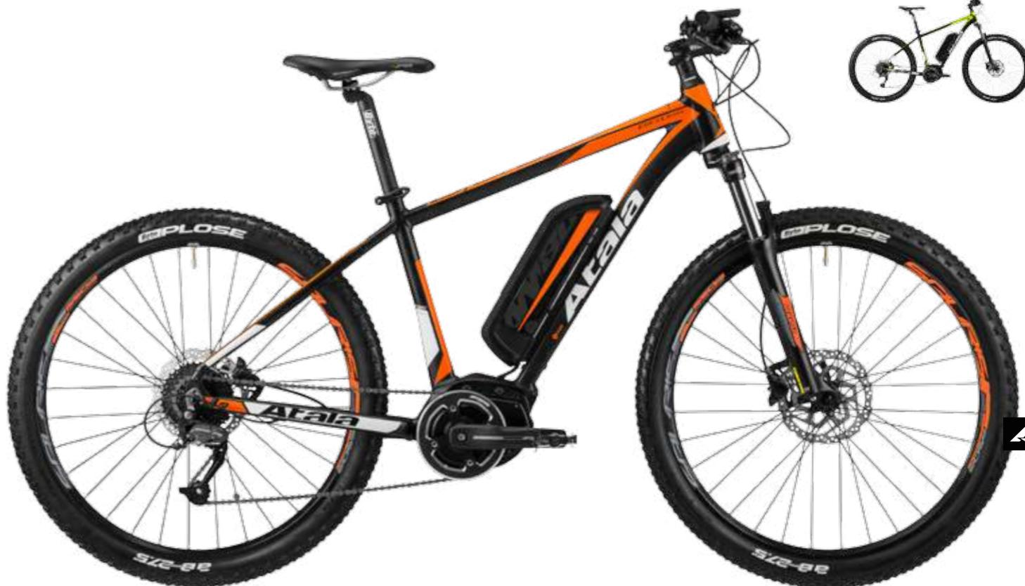
**FRAME** Alu 27.5", custom tubing, tapered, Internal Routing, Forged interface
