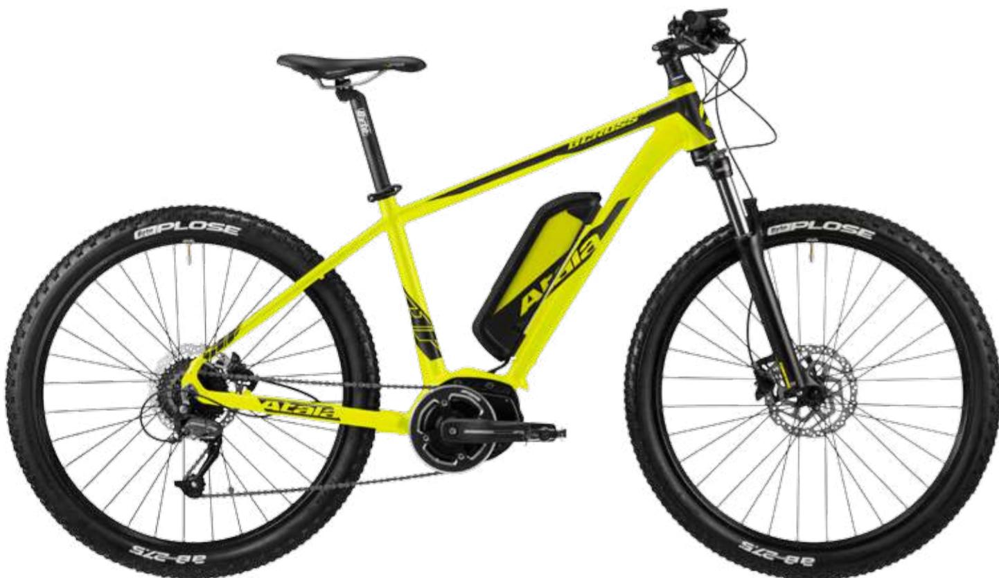
**FRAME** Alu 27.5", hydroformed, custom tubing, tapered, Internal Routing, Forged interface
