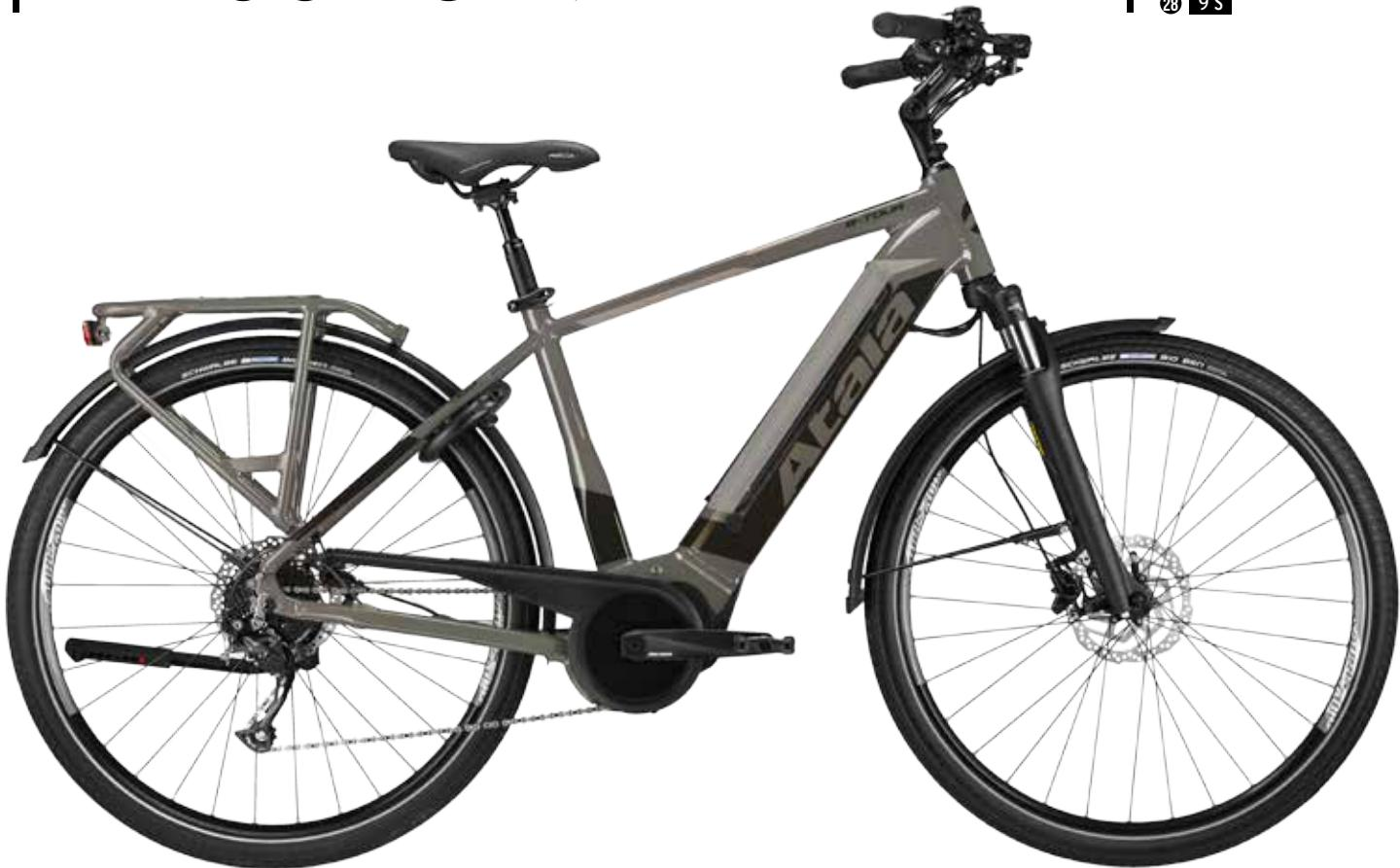
**FRAME** Alu 700C, hydroformed, integrated battery, custom tubing, Internal routing, Forged interface
