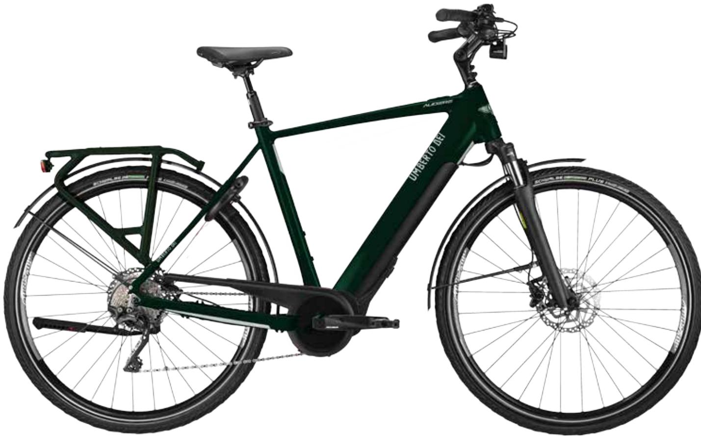
**FRAME** Alu, hydroformed, smooth welding, Post mount disc brake, Internal routing, tapered, 12x142 mm
