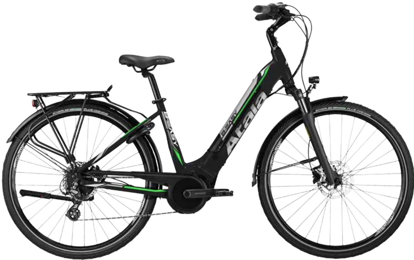
**FRAME** Alu 700C, hydroformed, easy access, integrated battery, custom tubing,
