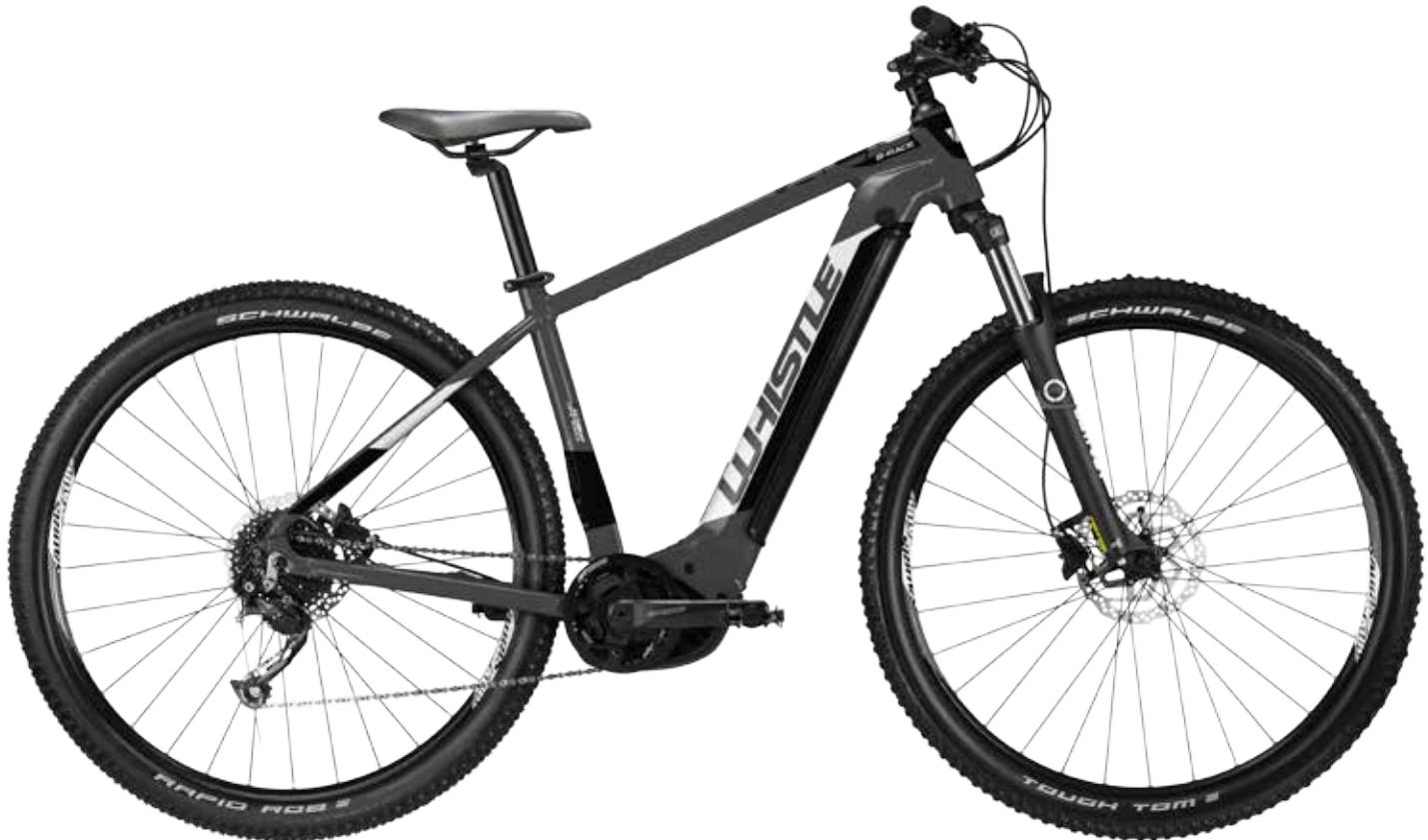
**FRAME** Alu 29", hydroformed, integrated battery, tapered, Internal routing,
