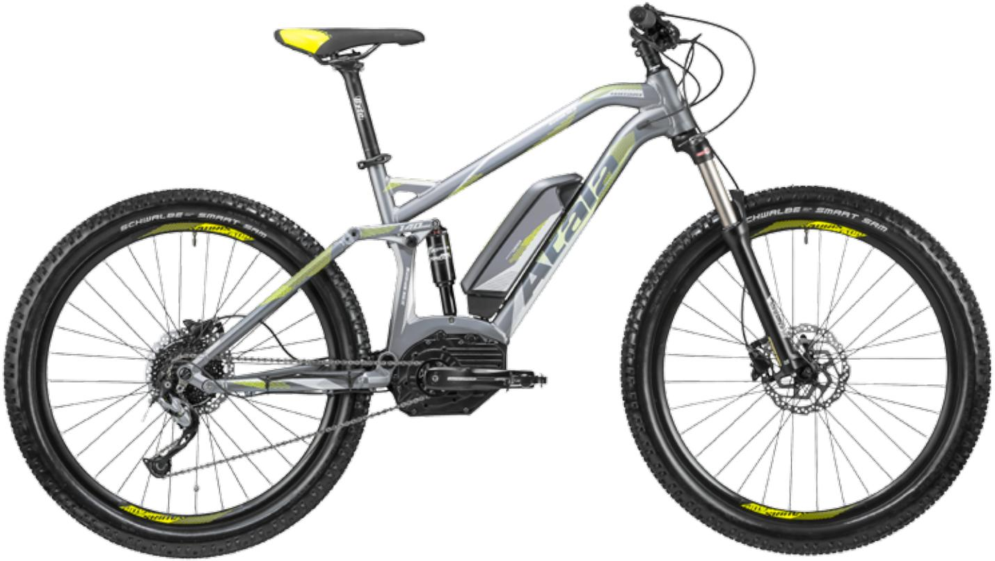
**FRAME** Alu 27,5"+, hydroformed, tapered, Rear travel 140 mm, 12x148 mm, Gravity casting interface
