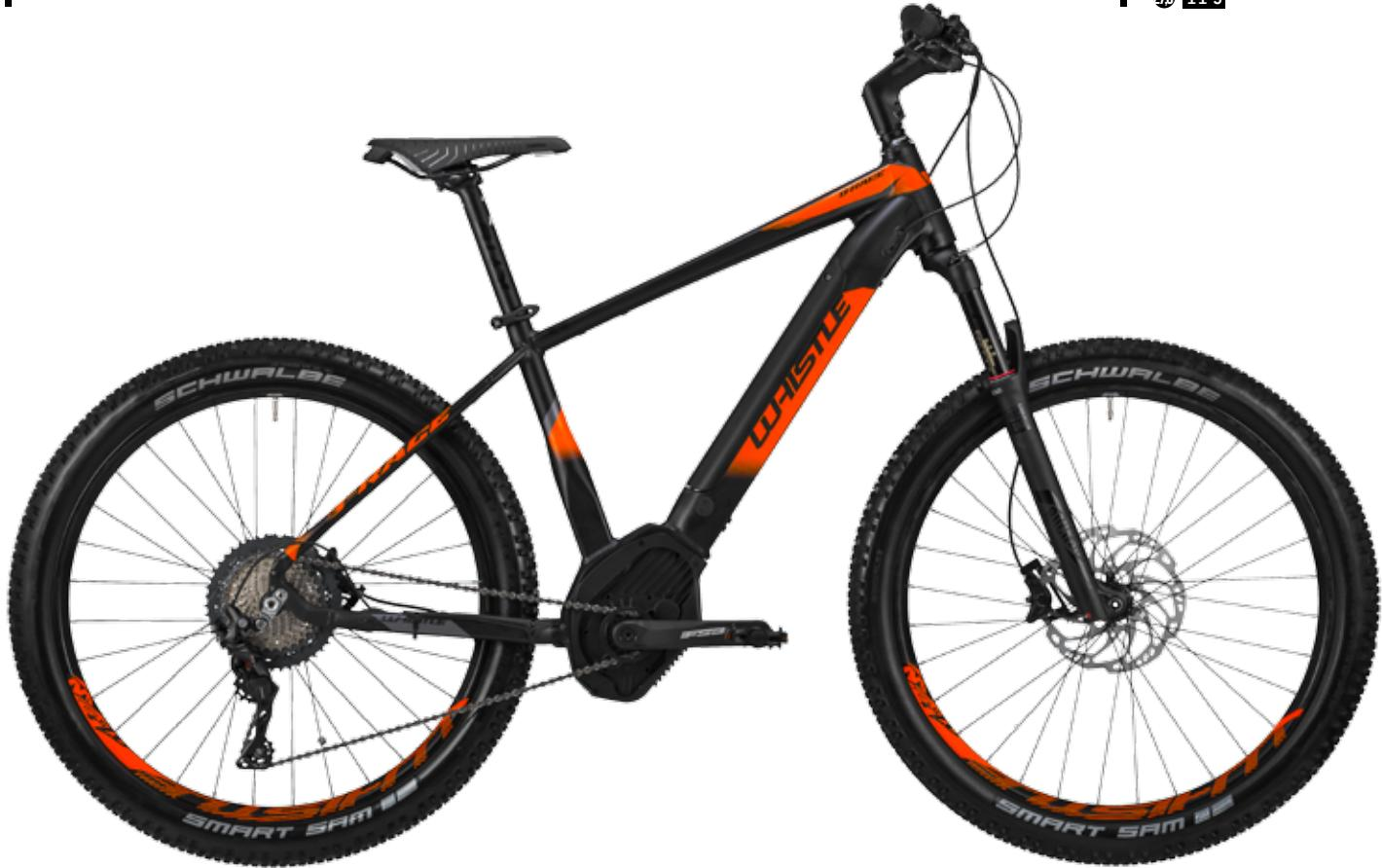
**FRAME** Alu 27,5"+, hydroformed, integrated battery, tapered, 12x148 mm
